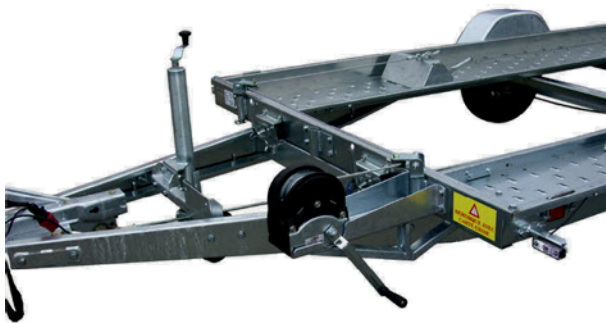
Winch with mounting bracket
